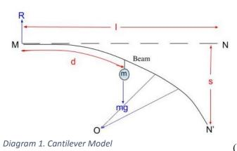
Consider a cantilever, fixed at one end, M, and loaded at a distance(cm), d. The end, N, is depressed to N' and s or [N'-N] represents the vertical depression at the free end. Note that N may not be at the same height(cm) level as M. There can be an initial vertical depression before any external force is exerted on the cantilever. The force exerted downwards by load- mg (Newtons), is equally and oppositely opposed by reaction force, R, acting
